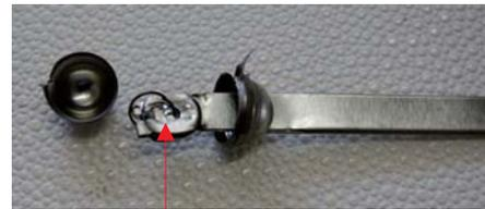
The internal structure, one spring perforation
